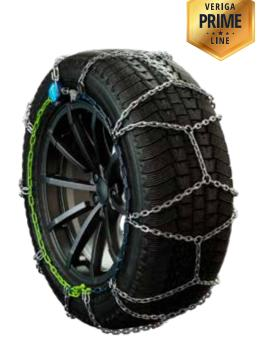
9 mm chain with automatic tensioning and centring of the chain. One patented self-tensioning and self-centring "STOP&GO" devices. Stopping the vehicle and tensioning the chain is not required.
